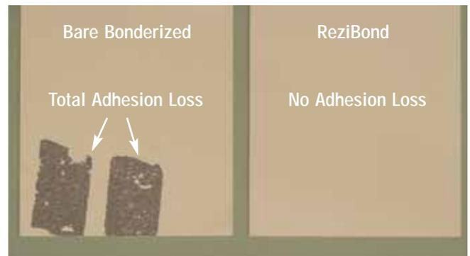
Samples of both products were also subjected to Gardner Impact testing where a weight is dropped from various heights, impacting the materials. As illustrated below, the adhesion of the paint was better to ReziBond product than to traditional bonderized.
